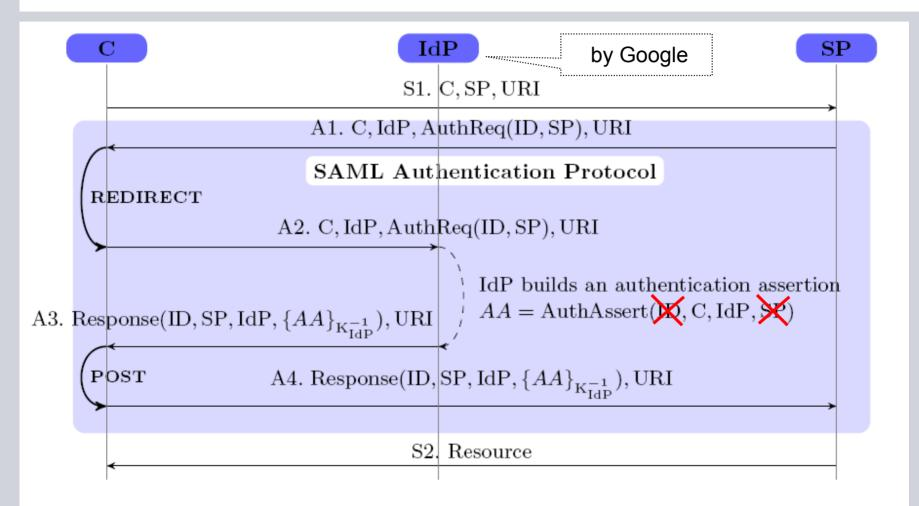
Fig. 1. SP-Initiated SSO with Redirect/POST Bindings
