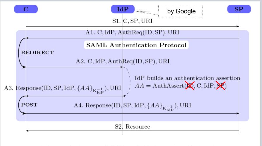
Fig. 1. SP-Initiated SSO with Redirect/POST Bindings
