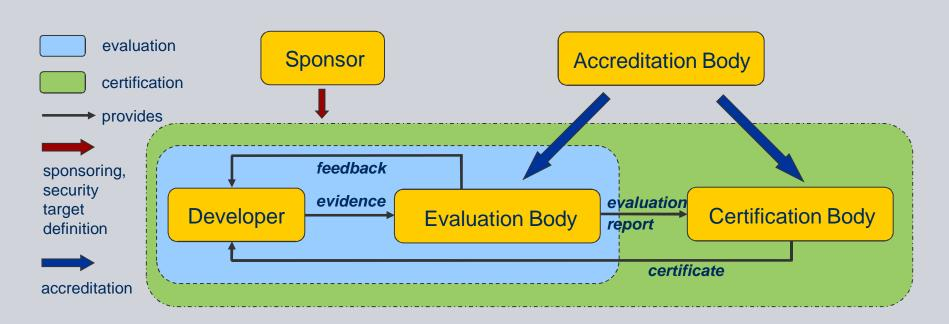
Certification according to the Common Criteria is a rather complex, time consuming and expensive process, providing systematic assurance.
