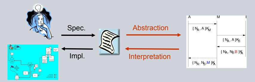
Improving the quality of the system specification Checking for the existence of security loopholes High-Level Protocol Spec. Language Model checkers (AVISPA tools)
