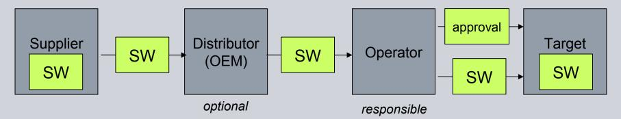
Transition from media-based (CD-ROMs etc.) to networked SW transport increases security risks due to transport over open, untrusted networks
