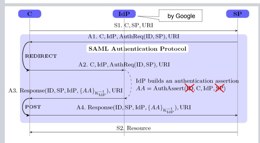
Fig. 1. SP-Initiated SSO with Redirect/POST Bindings
