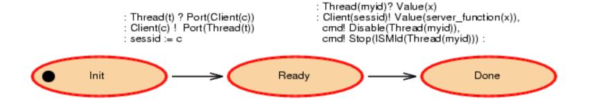
The thread receives the client port, sends its own port to the client, receives a value, transforms it, and sends it back to the client. Finally, the thread disables its port and stops.
